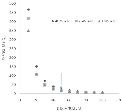
FIGURE 4. PLOT OF EXPOSURE (E) AGAINST DISTANCE (D) FROM THE SOURCE (ESB)
