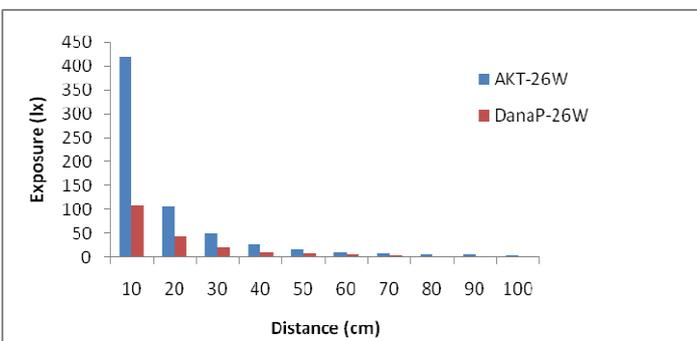
Figure 6. Comparison of Exposures of two products (manufacturers) of the same wattage
