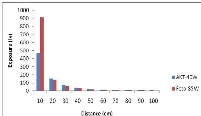
Figure 7. Comparison of two products (bulbs) of different wattages
