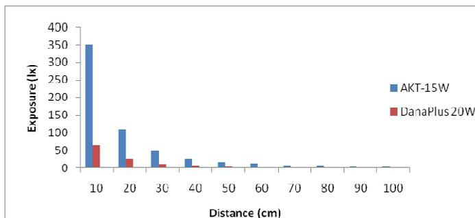
Figure 8. Comparison of two products (bulbs) of different wattages
