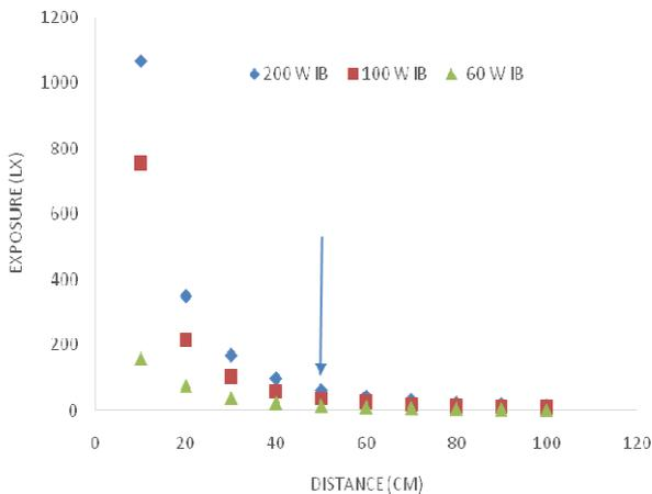
FIGURE 5: PLOT OF EXPOSURE (E) AGAINST DISTANCE (D) FROM THE SOURCE (IB)
