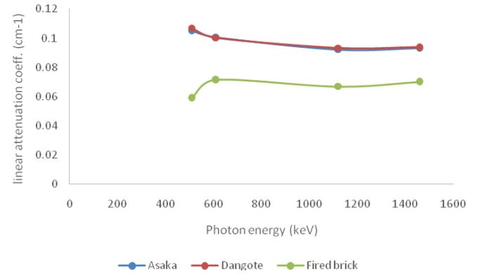
Figure 4: Dependence of Linear Attenuation Coefficient on Photon Energy
