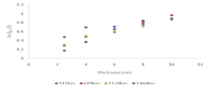
Figure 2: Determination of Linear Attenuation Coefficient of Concrete from Dangote Cement
