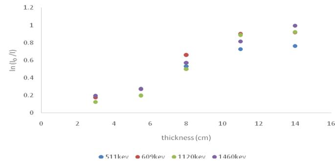
Figure 3: Determination of Linear Attenuation Coefficient of Fired Brick
