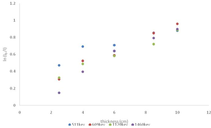
Figure 1. Determination of linear attenuation coefficient of concrete from Asaka cement
