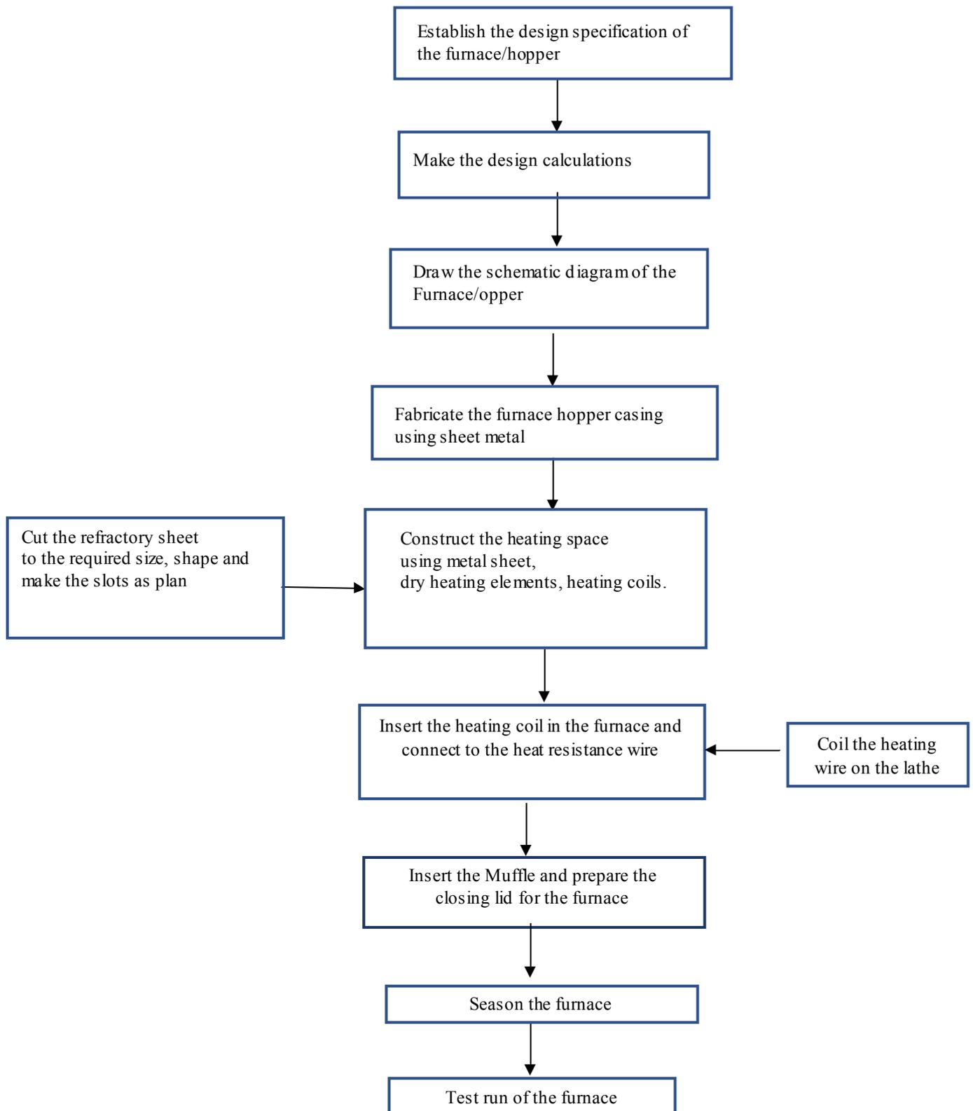
**Figure 8: Workflow in the Fabrication Process of the Furnace**
