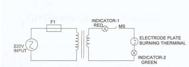
Figure 3: The circuit diagram of the needle burner
