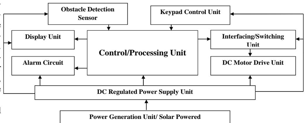
Figure 1: Block diagram of the main electrical system model
