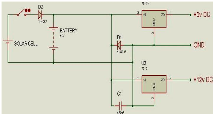
Figure 4: Power Supply Unit
