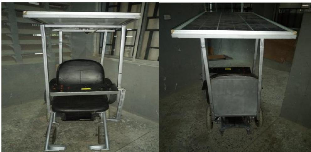
Figure 5: Picture of the Fabricated Solar Powered Wheelchair (back and front views)
