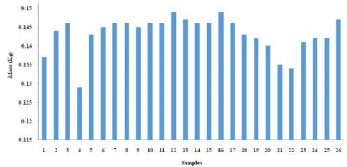
**Figure 2: Mass (Kg) of Samples after 28 Days**
