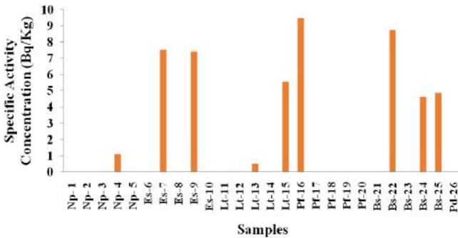
Fig. 5: Specific activity concentration of <sup>232</sup>Th in samples
