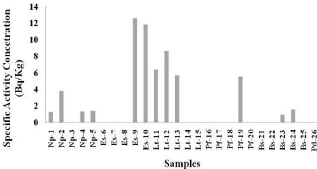
Fig. 6: Specific activity concentration of <sup>238</sup>U in samples
