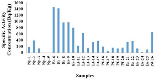
Fig. 4: Specific activity concentration of <sup>40</sup>K in samples
