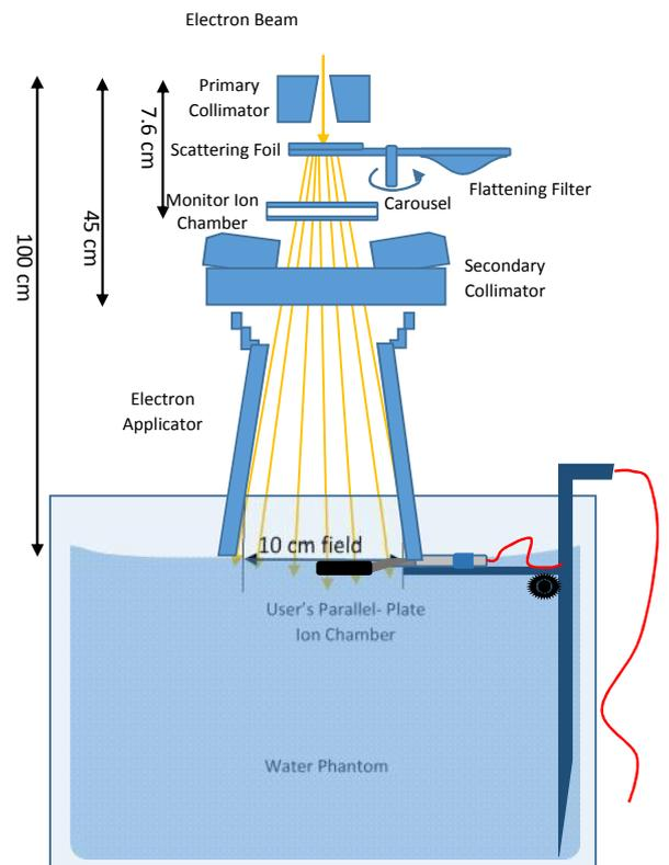
Figure 1b: LINAC beam calibration setup for Electron beam mode
