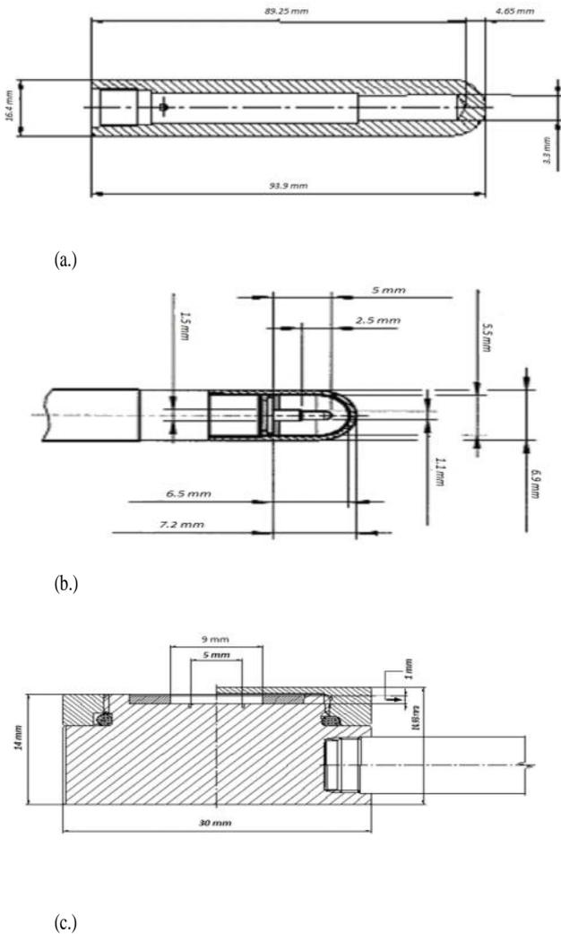
**Figure 2: The User Ion Chambers at the Radiotherapy Facility (a.) the PTW 30013 Farmer IC (b.) the PTW 31010 Semi-Flex IC and (c.) the PTW-3405 Advanced Markus IC with geometrical dimensions in mm**
