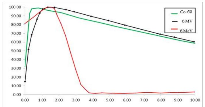
Figure 16: The Percent Depth-Dose Profile of the Co-60, 6 MeV and 6 MV Beam Qualities from Monte Carlo Calculation
