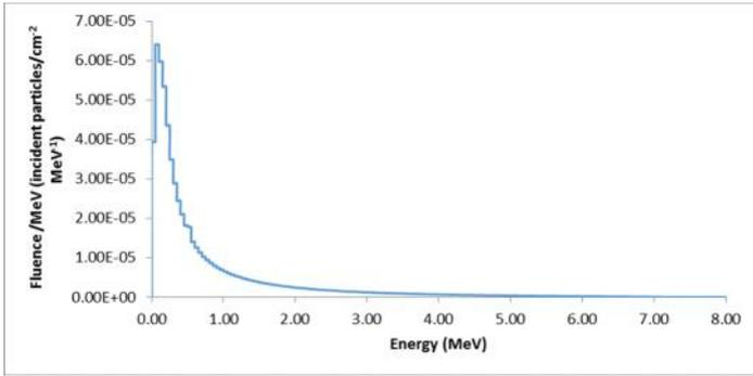
Figure 11: The Central-Axis Energy Spectral Distribution for 6 MeV Beam Phase Space showing Photon Particle Distribution at Low Energies
