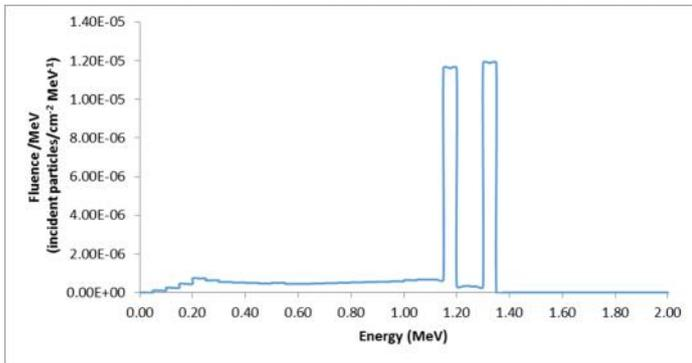
**Figure 7: The Central Axis Energy Spectral Distribution for the Cobalt-60 Beam Phase Space showing the Prominent 1.173 MeV and 1.332 MeV Gamma Photo-peaks.**
