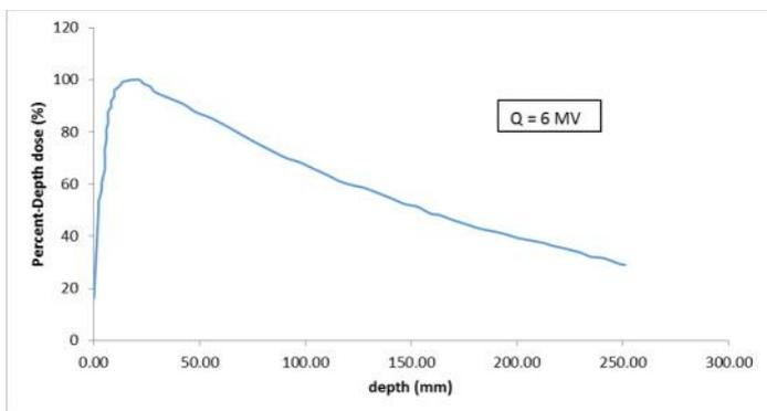
Figure 13: The Percent Depth Dose Profile of a 6 MV Beam for the Farmer IC from Monte Carlo Calculation at 10 x10 cm<sup>2</sup> Treatment Field and 100 cm SSD
