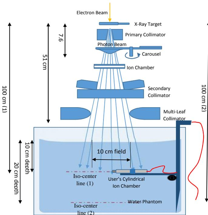
Figure 1a: LINAC beam calibration setup for photon beam mode based on  $TPR_{20,10}$  index, which depend on the two iso-center lines (1) and (2)
