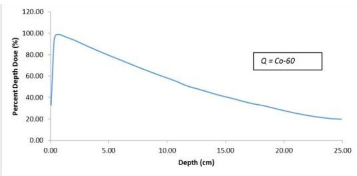
Figure 12: The Percent Depth Dose Profile in the Farmer IC of a Co-60 Beam from Monte Carlo Calculation at 10 x10 cm<sup>2</sup> Treatment Field and 100 cm SSD
