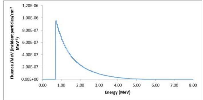
**Figure 9: The Central-Axis Energy Spectral Distribution for 6 MV Beam Phase Space Showing Electron Particle Distributions at Low Energies**
