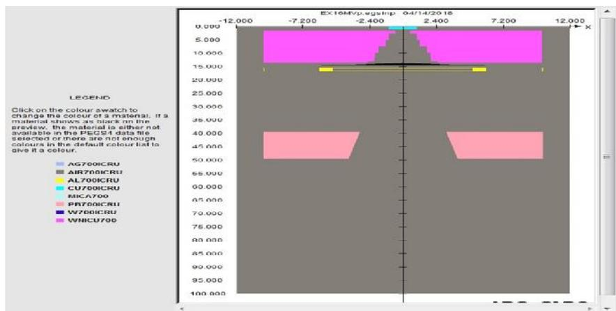
Figure 5: The Treatment Head Preview Generated from the Input Files Modified for Elekta Precise LINAC Machine in Electron-Therapy Mode
