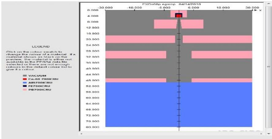
Figure 4: The Treatment Head Preview Generated from the Input Files Modified for Theratron-780 Co-60 Machine
