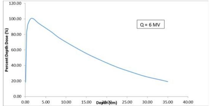
Figure 14: The Percent Depth Dose Profile in the Semi-Flex IC of a 6MV Beam from Monte Carlo Calculation at 10 x10 cm<sup>2</sup> Treatment Field and 100 cm SSD
