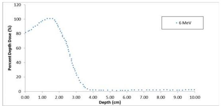
Figure 15: The Percent Depth Dose Profile of a 6 MeV Beam from Monte Carlo Calculation at 10 x10 cm<sup>2</sup> Treatment Field and 100 cm SSD of the Advanced Markus PTW 34045
