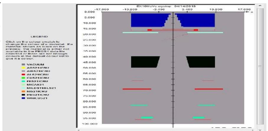
Figure 6: The Treatment Head Preview Generated from the Input Files Modified for Elekta Precise LINAC Machine in Electron-Therapy Mode
