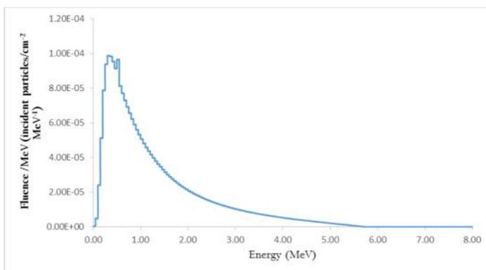
**Figure 8: The Central-axis Energy Spectral Distribution for 6 MV Beam Phase Space showing Photon Particle Distribution at Low Energies**
